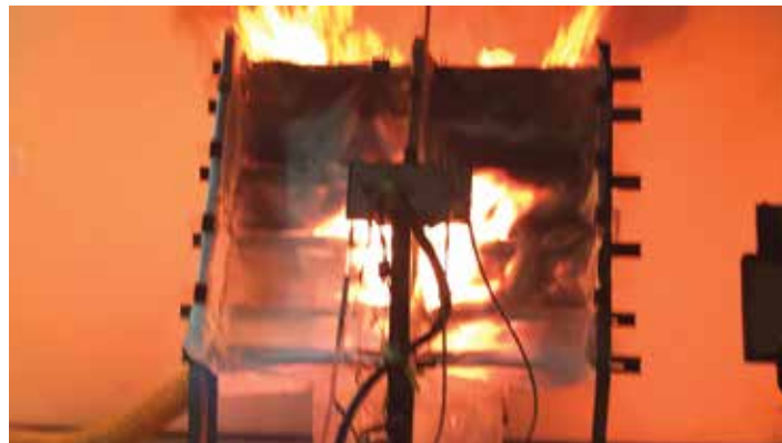
Figure 2. Flame Propagation Test as per FAR25.856-a : AF-10 fabric one layer, when tested per FAR25.856-a, after 4 min exposure, shows no after flame and no flame propagation
