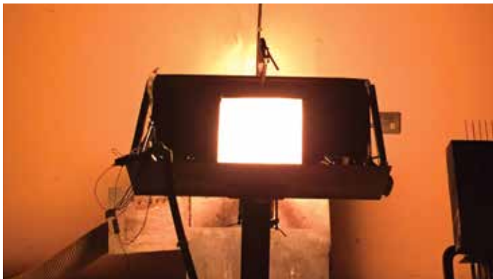
Figure 1. Flame Propagation Test as per ISO2685 : AF-10 Fabric one layer, when tested per ISO2685 conditions, after 15 min exposure there is no flame penetration and no after flame
