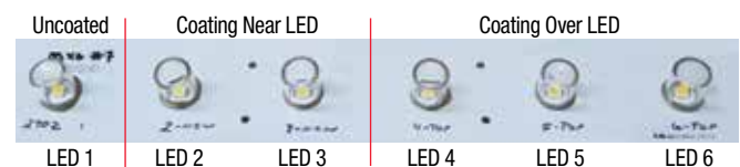
Figure 2. Cree LED test board after Novec coating and glass cap applied.
