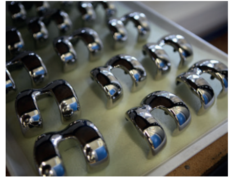
Parts are tested to ensure there are no traces of oils or compounds remaining.
