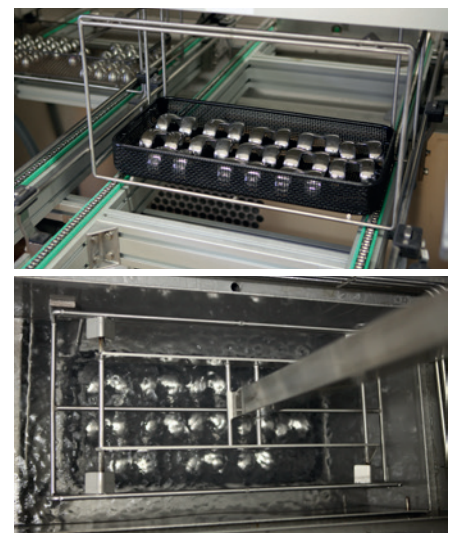
Parts are pre-cleaned and then immersed in 3M™ Novec™ 72DA Engineered Fluid for rigorous cleaning
