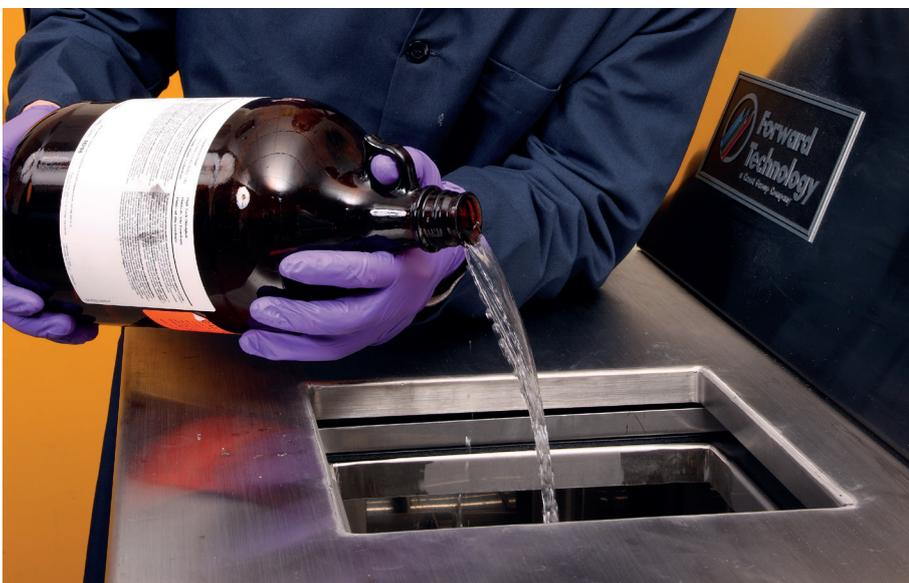
3M™ Novec™ Engineered Fluids are designed to balance performance with favourable environmental and worker safety properties. They are available for a wide variety of applications, including heat transfer, cleaning, testing, and lubricant deposition. Novec fluids offer excellent dielectric properties; wide range of boiling points; good materials compatibility; low toxicity and non-flammability; low global warming potential; and zero ozone depletion potential.
